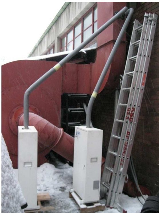
Figure 1: Sampling of large quantities of particulate matter with two Digital high-volume samplers from the laboratory main exhaust duct acting as an improvised full-flow dilution tunnel.
