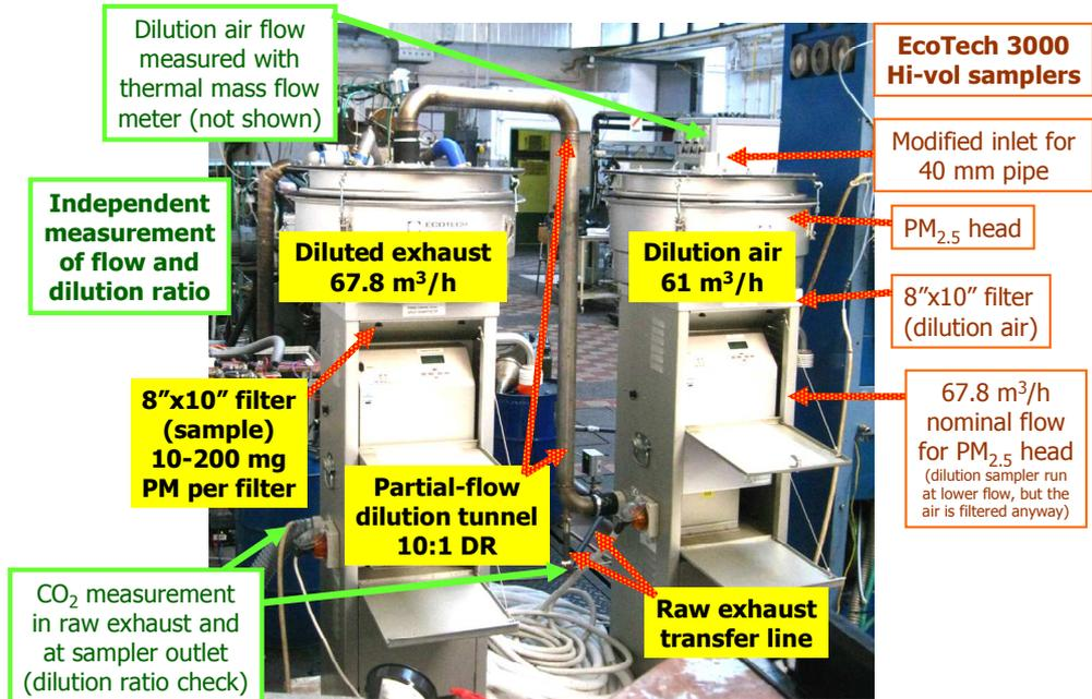
**Normal operation - filter capacity not reached**
